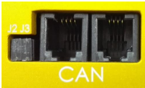
CAN BUS Socket and Jumpers (J2, J3)
